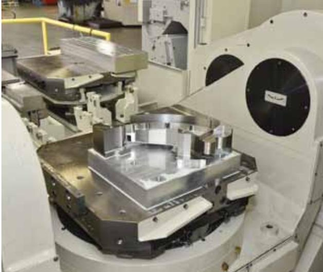
***Dual-pallet system on the two trunnion-style Mitsui Seiki HU63A-5X machines enable the titanium stock to be loaded while the workpieces are being machined.***
